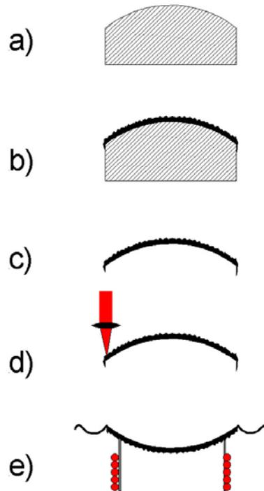
Fig.1: Processing steps to prepare dome shaped CVD diamond tweeter membranes. a) preshaped silicon substrate. b) substrate after deposition of CVD diamond. c) diamond dome after separation from the substrate. d) laser cutting of diamond dome. e) diamond membrane assembled with surround and voice coil former.
