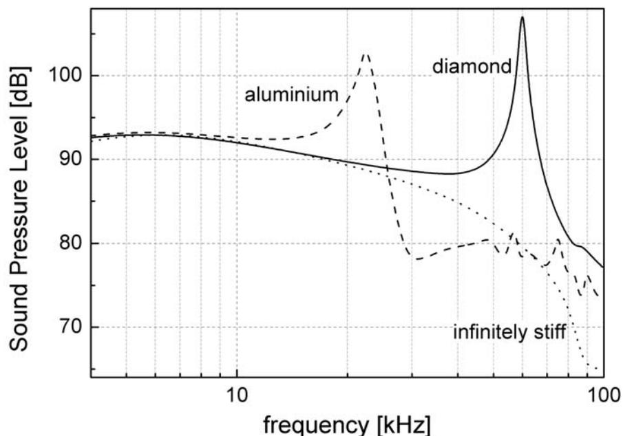
Fig.5: SPL vs. frequency for an aluminium, a diamond and an infinitely stiff membrane, all of the same mass.
