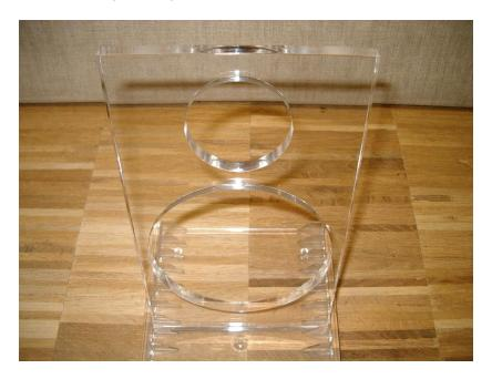
Material thickness should be at least 8mm, metal or acrylic will do nicely but it works as well with MDF or solid wood. Plywood is not recommended.
