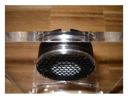
Align the driver in your frontplate with the holes in horizontal direction and the driver surface (not the protection grid!) in line with your speaker front.
