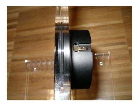
In this transparent acrylic frontplate you can see the perfect seal after tightening the two screws. Do not use too much force, light hand tightening will be enough.
