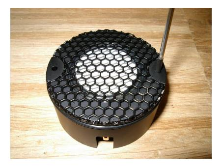
Tightening the screws will give a perfect seat for the driver. It will be air tight without any rigid connection to the frontplate. Note the shrink tube on the Allen key to prevent scratches on the driver surface.
