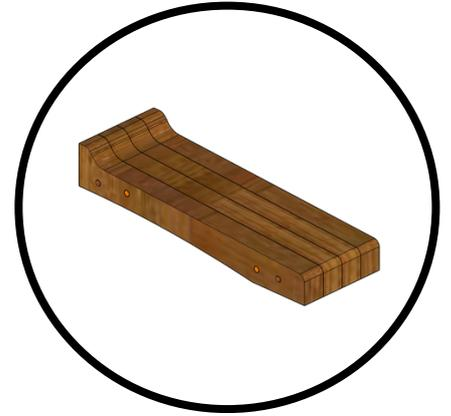
*Glue Component, align with 5" Dowels. Then flush cut.*
