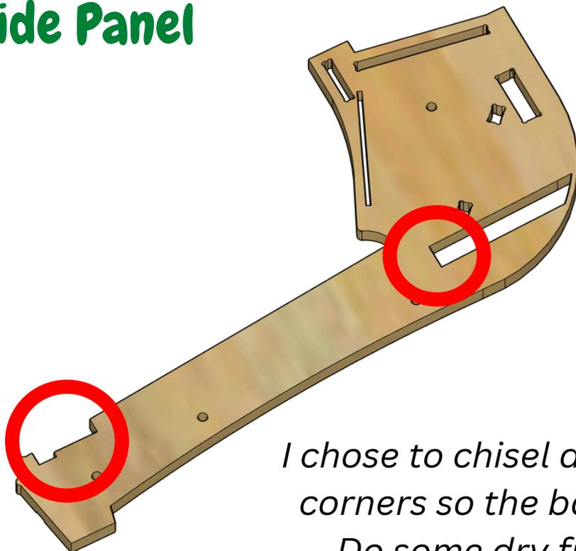
*I chose to chisel and file down these two corners so the balls would flow easier. Do some dry fitting to test things.*
