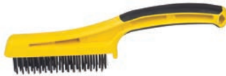
46802 Carbon Steel Wire Stripping Brush Brush area measures 3/4" x 4-3/4" with .35mm bristles. Overmold handle.
