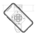
8 Twist device until a click is heard to ensure a secure lock. Once locked in place, make sure the mount is secure.
