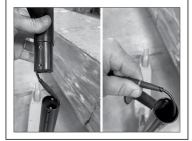
Using a flat screwdriver, remove the grommet at the bottom of the stem.
