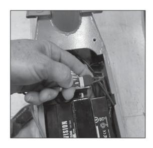
Using a Phillips screwdriver, remove two (2) screws from the battery bracket. Remove the battery bracket and set aside. Remove the old/used battery and replace with new battery.
