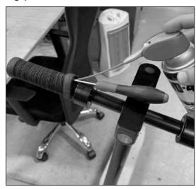
Repeat the steps on the other side, clean handlebars and grips before installing new grips.
