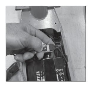
Using a Phillips screwdriver, remove two (2) screws from the controller bracket. Remove the bracket and controller from the unit and set aside.
