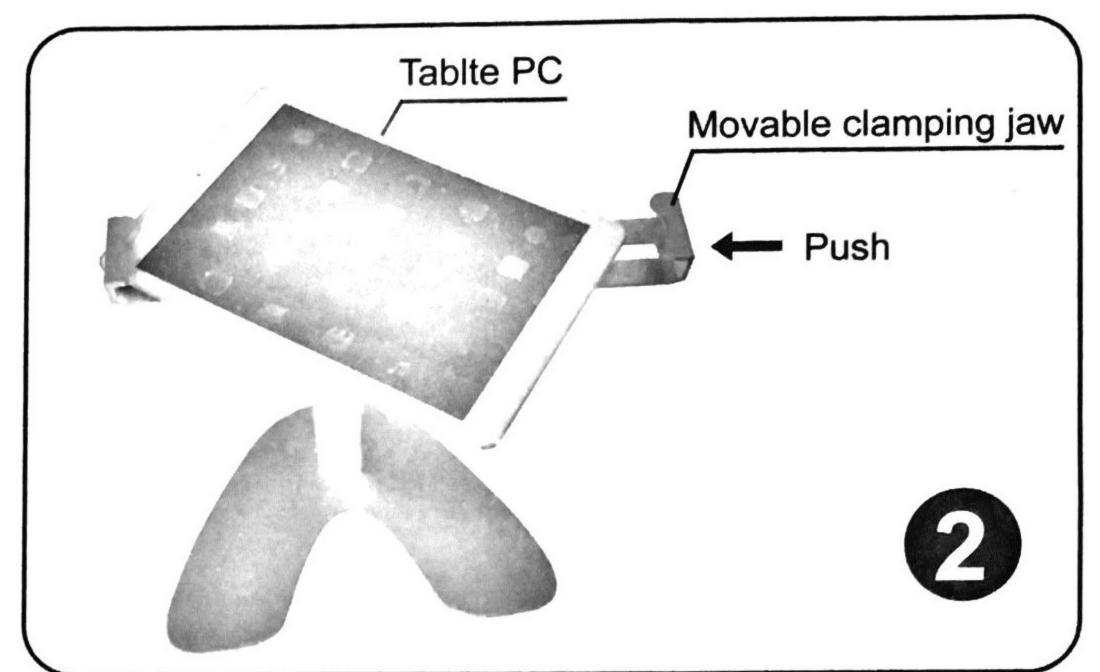
3)Push the lock catch on the holder back to catch the movable clamping jaw after the Tablet PC is clamped by the jaw and then turn the key to lock it.
