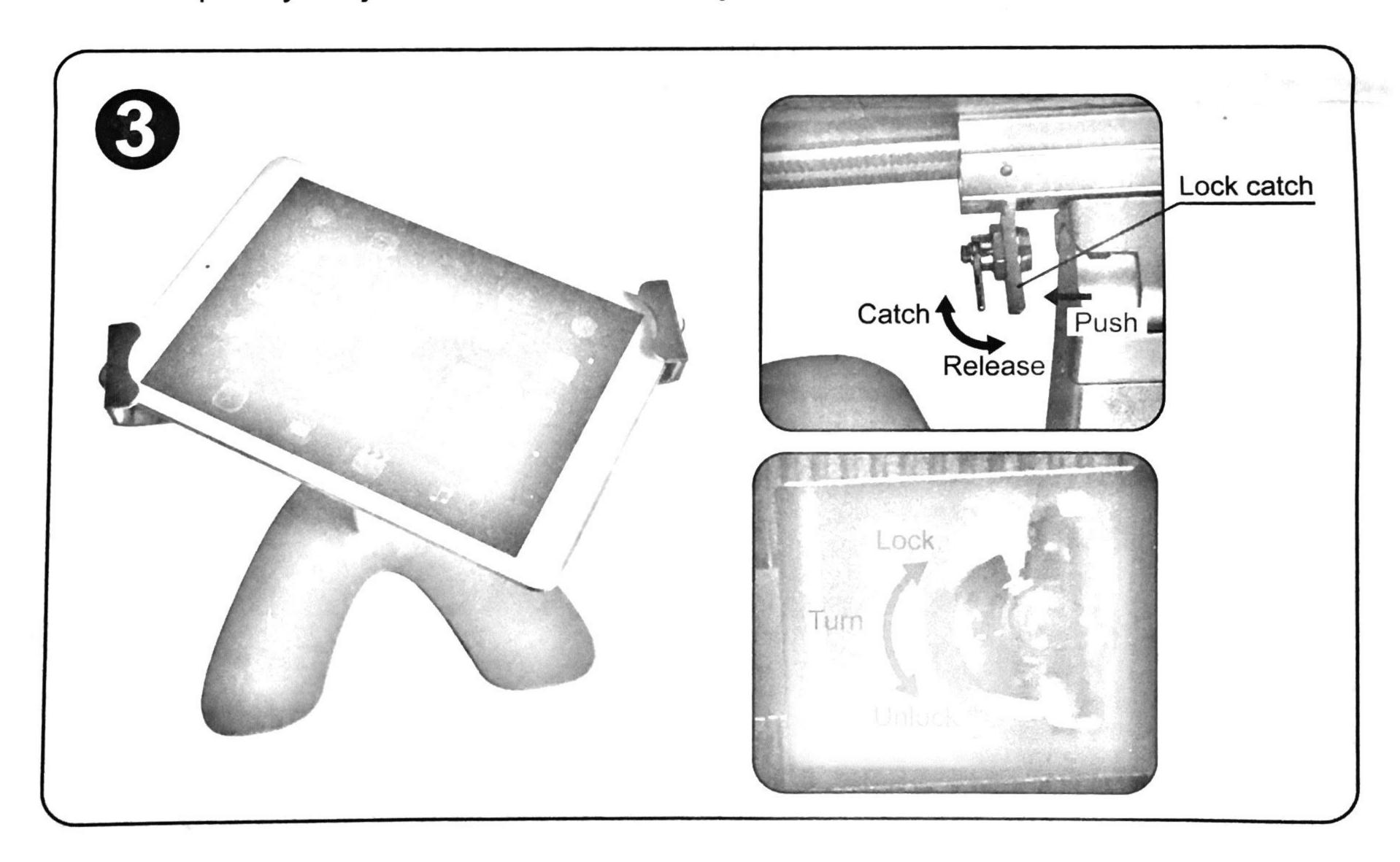
4)To avoid the Tablet PC dropping, please make sure the Tablet PC has been clamped securely before adjusting the holder angle you need.
