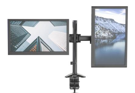
The adjustable arm offers -90°/+35° tilt, 180° swivel, 360° rotation, and height adjustment along the center pole.
