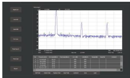
Use the provided EMI software (available for download at www.bkprecision.com ) to configure the spectrum analyzer, perform prescan, peak search, final scan and generate reports of your pre-compliance tests.
