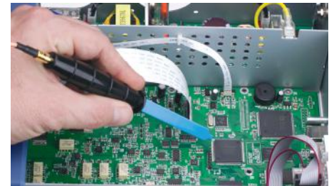
Use near field probes to help track down emissions.
