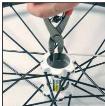
Using an internal circlip pliers, refit the two bearing retaining circlips by positioning them in the notches provided.
