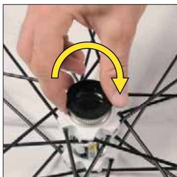
It is recommended that the Center Lock lock nut be mounted so as not to damage the hub body.
