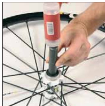
Using the press kit, remove the disc side bearing by the non-disc side.
