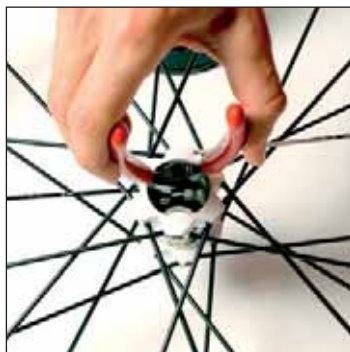
Using an internal circlip pliers, remove the two bearing retaining circlips.
