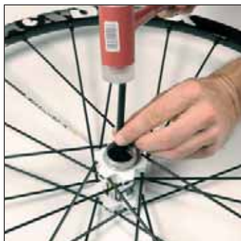
Remove the non-disc side bearing with the press kit.
