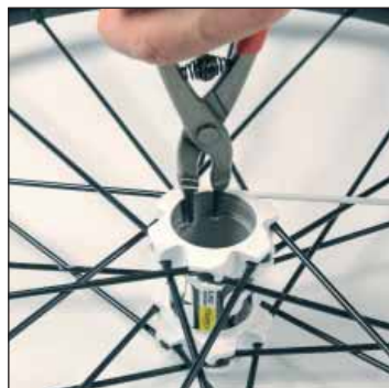
Using an internal circlip pliers, remove the two bearing retaining circlips.
