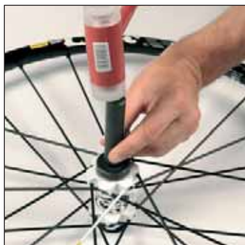
Introduce the non-disc side bearing with press kit 308 732 01.
