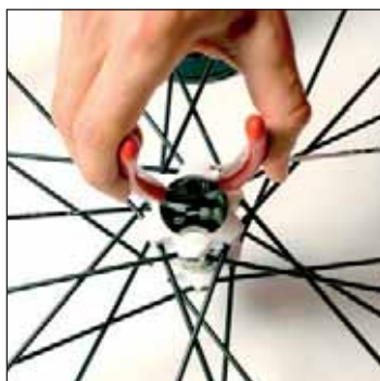
Using an internal circlip pliers, refit the two bearing retaining circlips by positioning them in the notches provided.
