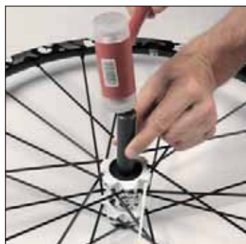
Using the press kit 308 732 01, introduce the new disc side bearing via the non-disc side.
