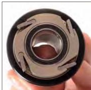
Center the internal spacer of the free wheel body, then slide the assembly onto the hub axle.
