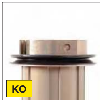
Remove the lip seal to clean or replace it, then refit it. Its lip must not come in contact with the free wheel body. Check that the base of the seal is flat against the entire free wheel body circumference.
