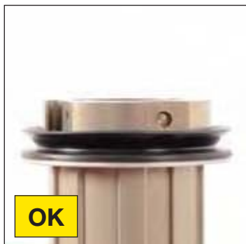
Remove the lip seal to clean or replace it, then refit it. Its lip must not come in contact with the free wheel body. Check that the base of the seal is flat against the entire free wheel body circumference.
