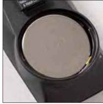
Refit the battery with the + side visible and close the battery cover.
