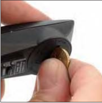
Open the battery cover and remove the battery.
