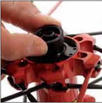
Unclip the non-disc side fork support.
