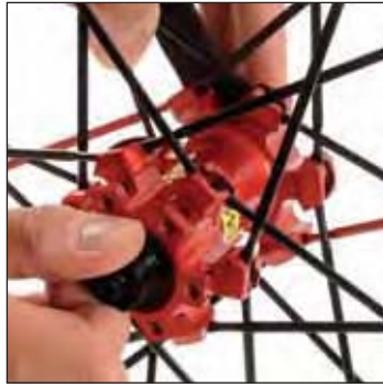
Hold wrench M40123 in place and loosen the axle with your fingers via the disc side.
