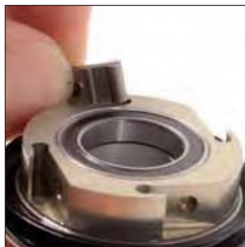
Grip the pawl-spring assembly between your thumb and left forefinger and slide it in the throat of the free wheel body. Check that the spring is housed correctly.
