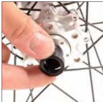
Unclip the non-drive side frame support.
