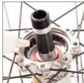
Clean the hub body and fill three ratchet teeth with oil M40122.
