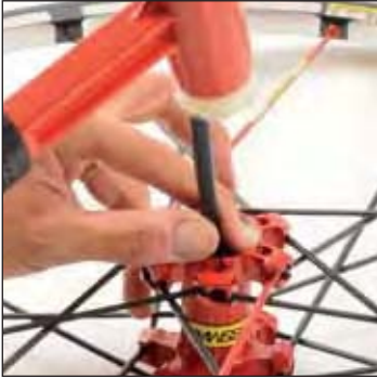
Use a bearing press kit to remove the bearings.
