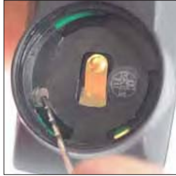
Press the contact switch set back from the base of the battery with a metal tip.
