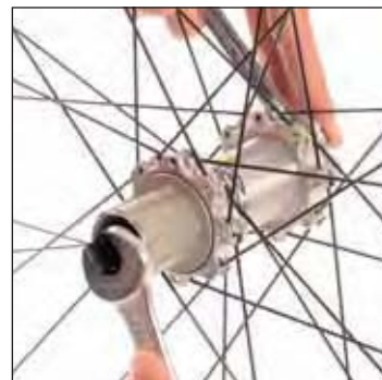
Holding the axle with the 14 mm open-end wrench via the non-drive side, tighten the drive side lock nut with the 17 mm open end wrench. (torque: 15 Nm maximum).
