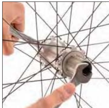
Holding the axle with the 14 mm open-end wrench via the non-drive side, loosen the drive side lock nut with the 17 mm open end wrench.
