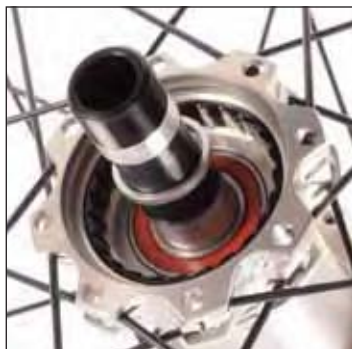
Check that the ITS4 spacer is in place before refitting the free wheel body.
