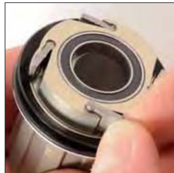
Slide the pawls in their groove to separate them from the free wheel body. Take care not to lose or damage the springs.
