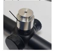
Finally fit the outer cap over the inner turret and gently tighten the  $3 \times M4$  grubscrews. If a small adjustment to zero is required, simply loosen the  $3 \times M4$  grubsrews, set zero and tighten back in position.
