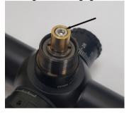
Fit the inner turret over the brass sleeve and gently tighten the 3 grub screws.
