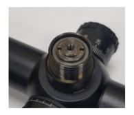
Fit the brass bush to the top of the turret spigot with M4 x12 bolt and lightly tighten ensuring the slot aligns and engages with the turret flats.
