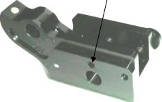
3. The grub screw fitted to the top of the loader arm allows the oring which grips the pellet to be adjusted for grip. Screw inwards to swell the oring and provide more grip.
