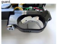
5. Take the spring and cap out of the original trigger and put them in the replacement trigger. Visually match the grub screw settings across to the new trigger. Loosely set the trigger post to the position of the original trigger to assist assembly. Do not tighten.
