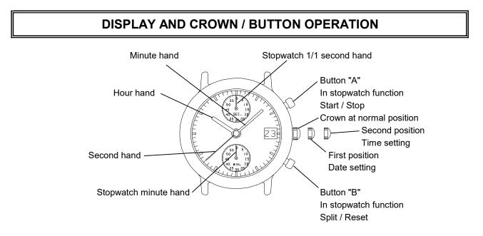
\*The measurement time is indicated by the stopwatch hands that move independently of small second hand.
