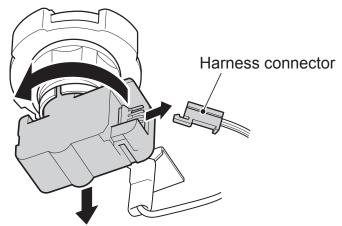
3 Pull out the LED lamp from the illuminated switch.
