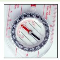
2) While holding the compass level, and directly in front of you, rotate your body with the compass until the North end of the needle (usually Red) is pointing to your declination value on the declination scale (-4 or 4 degrees Westerly in this case).
