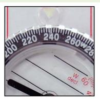
3) Now you can read your True North direction of travel to the object by reading the location where the bezel crosses the reading line inside the bezel (239 degrees in this example).
