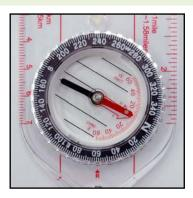
2) Rotate the bezel until the North end of the needle (usually Red) is pointing to your declination value on the declination scale (In this case pretend your declination is -4 or 4 degrees Westerly)
