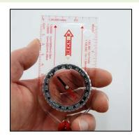
1) Hold the compass level, and directly in front of you, with the direction of travel arrow (The Treknor logo on the T580 Orienteer) pointing to the object ahead.
