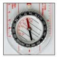
1) Rotate the bezel on your compass until the reading line is at the desired direction. (In this case, pretend you want to head at a bearing of 55 degrees).
