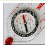
2) While holding the compass level, and directly in front of you, rotate your body with the compass until the North end of the needle (usually Red) is pointing to the "N" of the bezel (located at the 0/360 degree location on the bezel).
