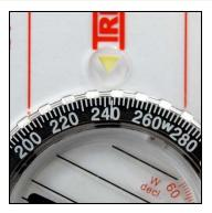
3) Now you can read your direction of travel to the object by reading the location where the bezel crosses the reading line inside the bezel (243 degrees in this example).
