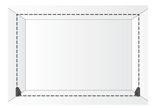
Then continue with the 2 ceiling corner cable anchors. Install each into the top plate in the same manner, with tapered end pointing down.
