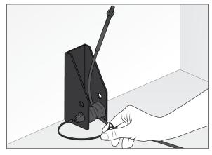
Connect the top and bottom cable ends together on each side via the turn-buckles and tighten just until cable system is taut. **Do not overtighten.**
