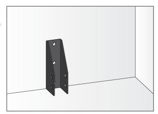
Make sure the corner cable anchor is level. Then mark the bottom angled hole and drill a pilot hole at a downward angle for the ¼" lag screw. Use one screw to secure it in place through the bottom angled hole into the bottom plate of the wall.
