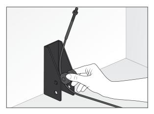
Secure the pulley wheel in place with the lynch pin through the lower hole closest to the floor.
