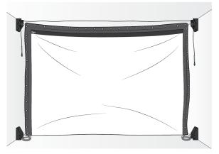
Loosely zip-tie the top 2 corners of the screen around the pulley wheel of the 2 ceiling corner cable anchors.
