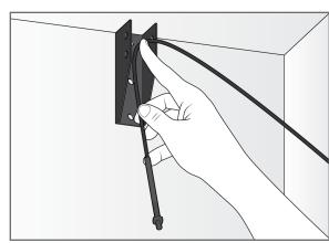
Secure the pulley wheel in place with a safety wire lynch pin through the lower hole.
