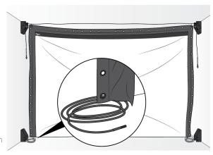
Take one end of the pre-threaded cable that runs through the bottom of the screen and press it into a floor corner cable anchor, then insert the pulley wheel.
