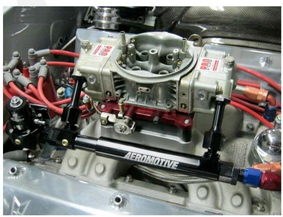
The fuel system's first priority is to keep the floats from running low enough to uncover the main jet, running the engine out of fuel. Traditional, static systems do a fair job of this. The second, more difficult priority is keeping the fuel level optimum in the bowl. It may not seem significant but the weight of fuel above the main jet does impact fuel flow through it, and therefore the air/fuel ratio of the engine under load.
