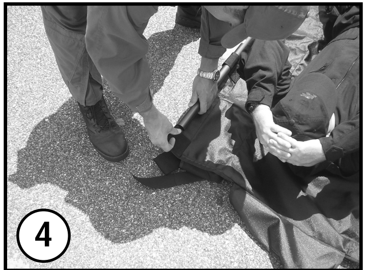
Insert other end of pole into end loop with elastic retaining band
