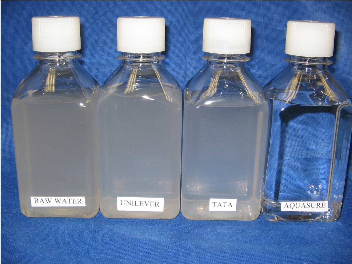
Comparison of raw water and after being filtered through Unilever Purit, Tata Swach and Eureka Forbes AquaSure
