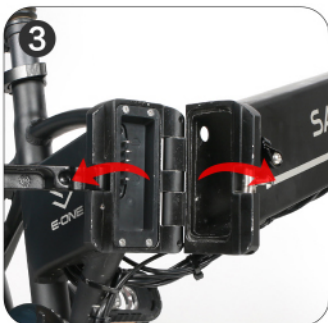
3 Fold open the ebike according to the direction
