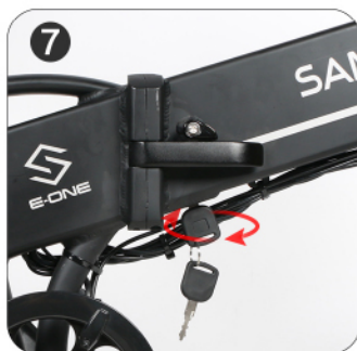
7 When you want to remove the battery, you need to unlock the battery according to the direction first. When the vehicle is powered on, you need to turn the two gears counterclockwise to unlock
