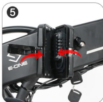
5 Insert the key into the key hole, turn clockwise to lock the battery, and then fold the frame
