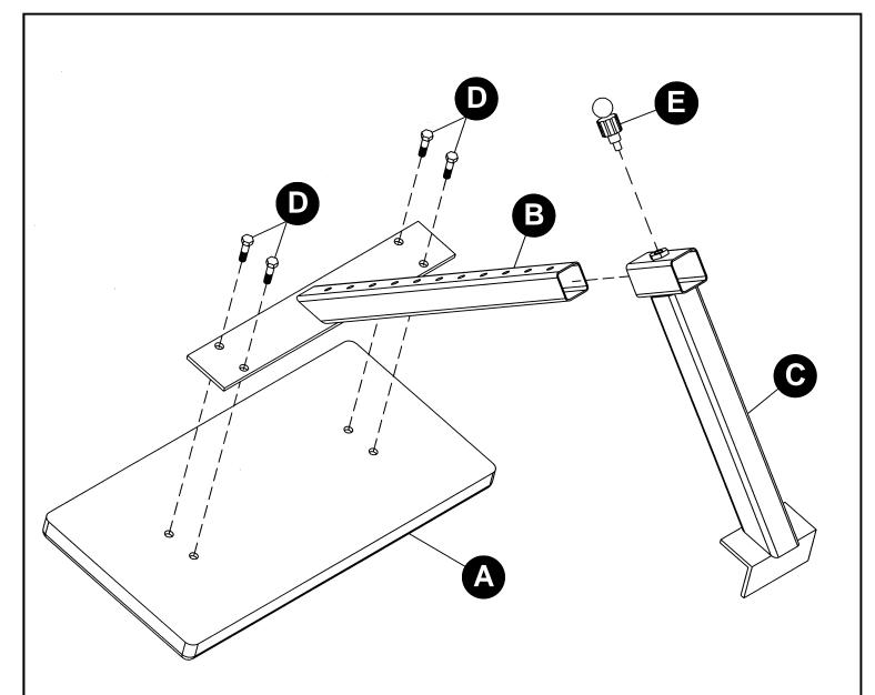
ASSEMBLE THE ARMREST PAD (A) TO THE ARMREST SUPPORT (B) USING THE M10 x 25MM BOLTS (D).
