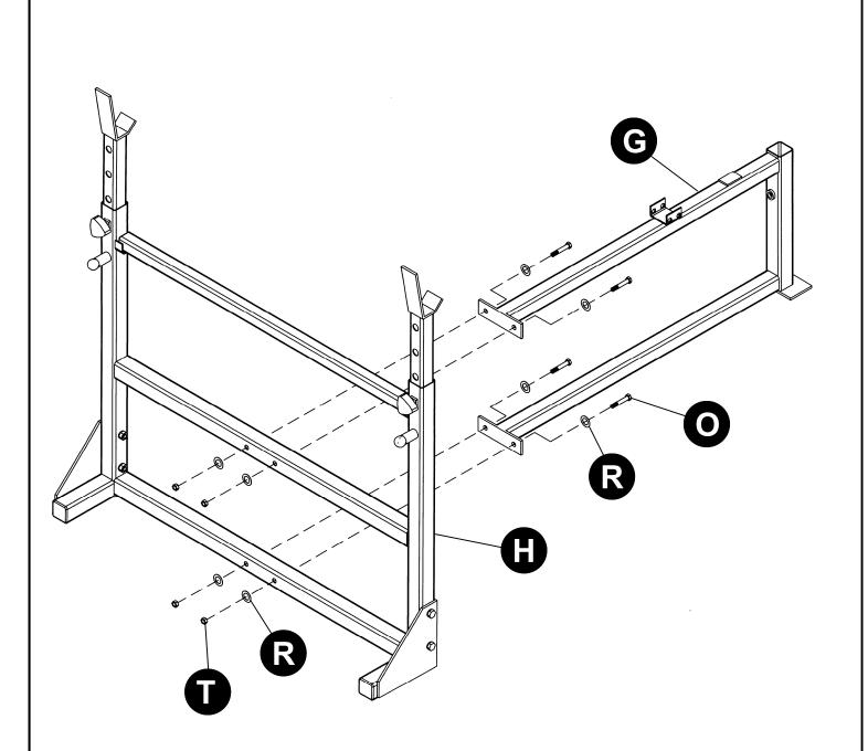
INSTALL MAIN FRAME (G) TO WEIGHT FRAME (H) USING M12 x 75MM BOLTS (O), M12 WASHERS (R), AND M12 LOCKNUTS (T).
