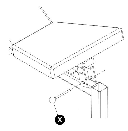
ROTATE SEAT TO DESIRED HEIGHT AND INSERT SEAT SUPPORT PIN **(X)** THROUGH SLOT. LOWER SEAT AND ALLOW PIN TO REST AGAINST MAIN FRAME. REMOVE SEAT SUPPORT PIN FOR FLAT POSITION.
