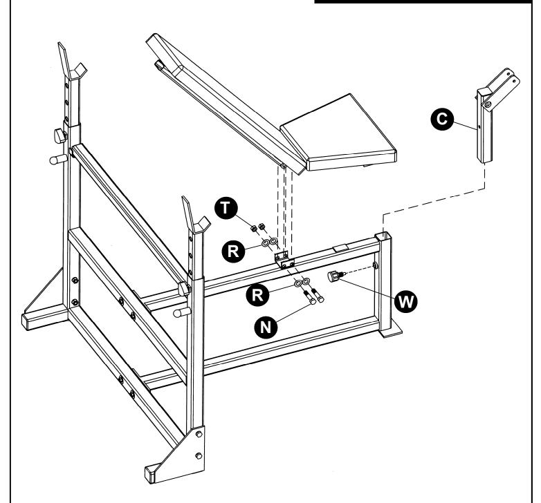
ATTACH THE BACKREST ASSEMBLY TO THE MAIN FRAME USING THE M12 x 79MM BOLT (N), THE M12 WASHERS (R) AND THE M12 LOCK NUT (T). ATTACH THE SEAT ASSEMBLY TO THE MAIN FRAME USING THE M12 x 79MM BOLT (N), THE M12 WASHERS (R) AND THE M12 LOCK NUT (T).
