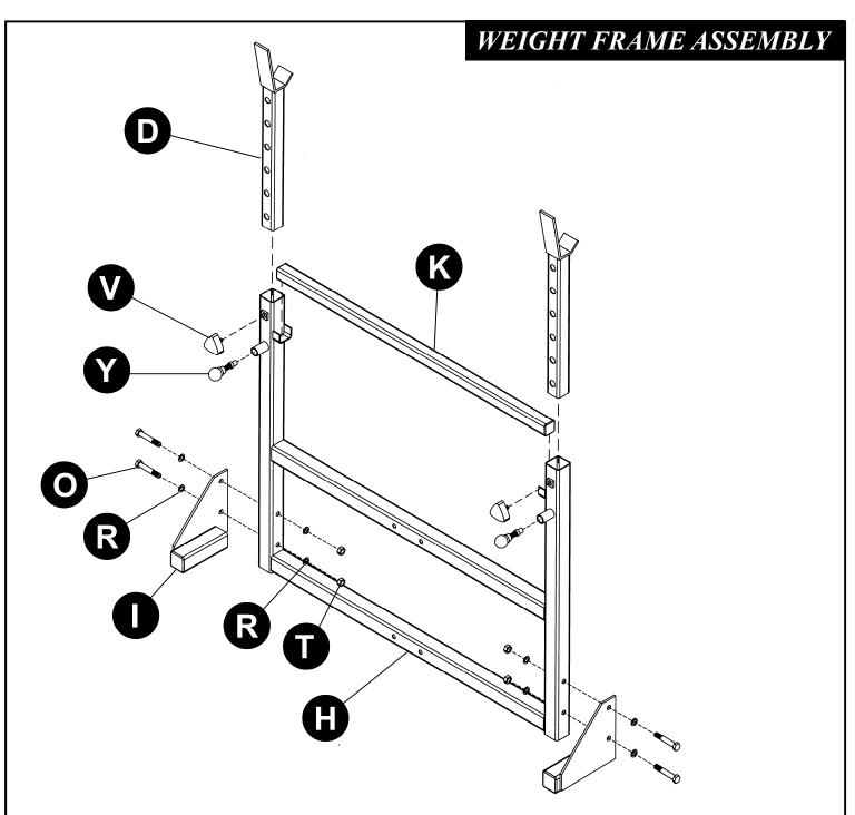
BOLT THE WEIGHT FRAME FEET (I) TO EACH SIDE OF THE WEIGHT FRAME (H) USING M12 x 75MM BOLTS (O), M12 WASHERS (R), AND M12 LOCKNUTS (T). DO NOT TIGHTEN NUTS AT THIS TIME.
