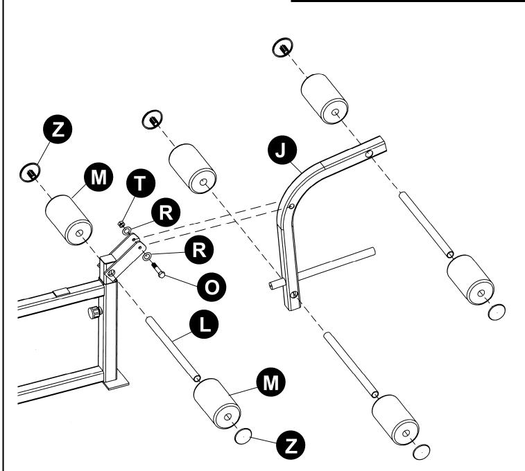
ATTACH THE LEG EXTENSION ARM (J) TO THE LEG YOKE USING M12 x 75MM BOLT (O), M12 WASHERS (K), AND M12 LOCKNUT (T).
