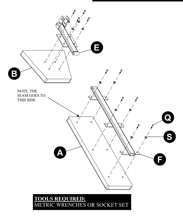
USE THE M10 x 25MM BOLTS (Q) AND THE M10 WASHERS (S) TO SECURE THE BACKREST (A) AND THE SEAT (B) TO THE SUPPORTS (E) AND (F). HAND TIGHTEN ALL BOLTS FIRST, THEN TIGHTEN SECURELY WITH WRENCH.
