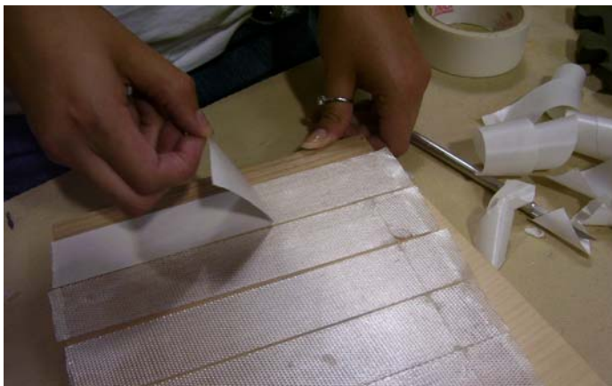
Figure 10 Use heavy duty double stick tape
