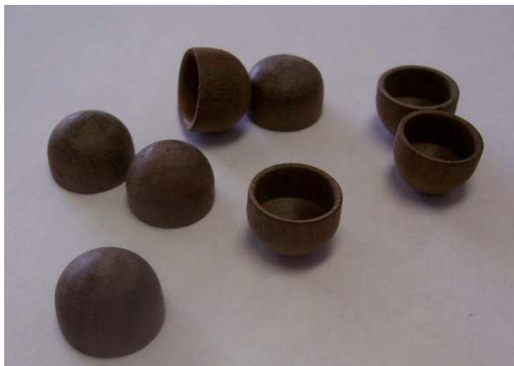
Figure 64 Turn nut covers by using a stub chuck on a lathe
