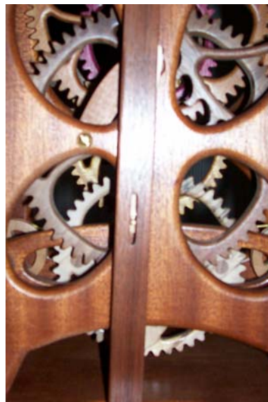
Figure 80 Swing of pendulum should be equal on each side of the center line. Adjust the escape lever arbor to make the adjustment.
