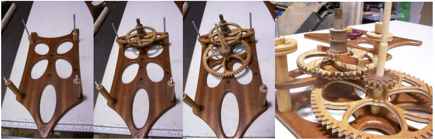
Add gear assemblies intermediate plate, ratchet and spacers with pulleys
