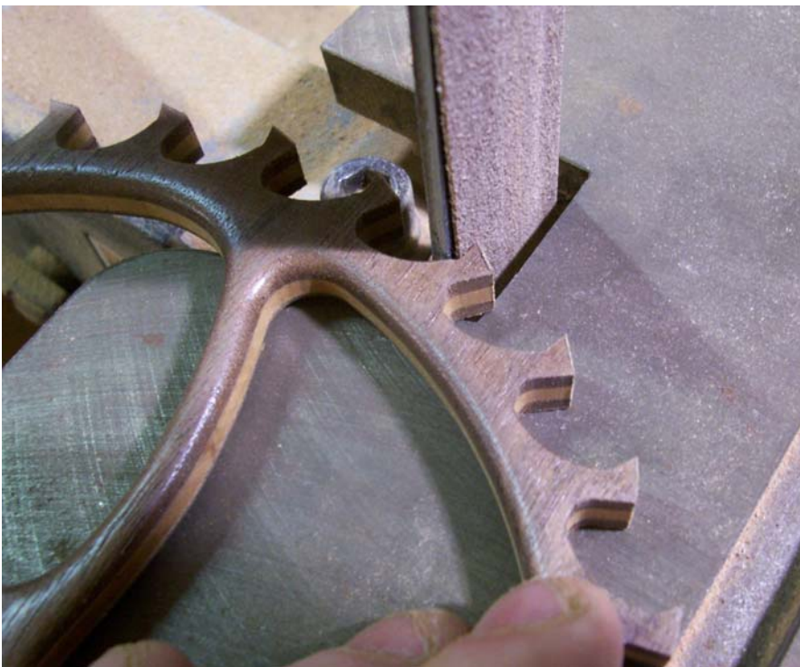
Figure 20 Sand the inside edge of each tooth on the #8 escape gear
