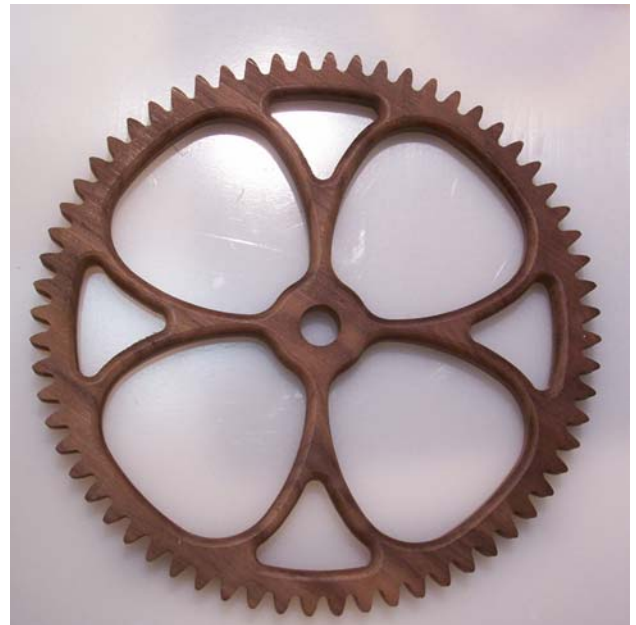
Figure 9 1/8" bit required to cut fine detail of teeth
