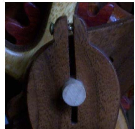
Figure 41 Small screw provides tension to hold hand in place.
