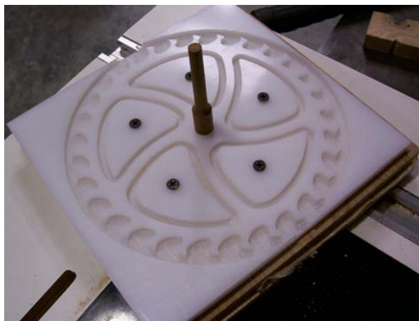
Figure 13 Gear blank with center dowel and sacrificial board ready for cutting.
