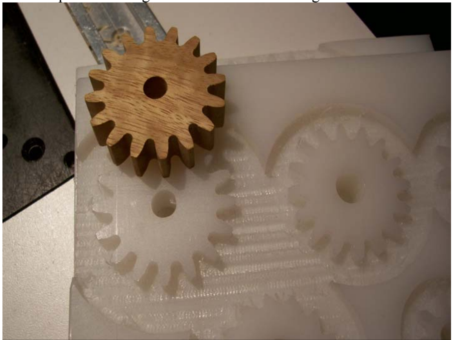
Figure 16 #17 16 tooth pinion has smaller center hole. These pinions are drilled to accept a small screw. See instructions in assembly section
