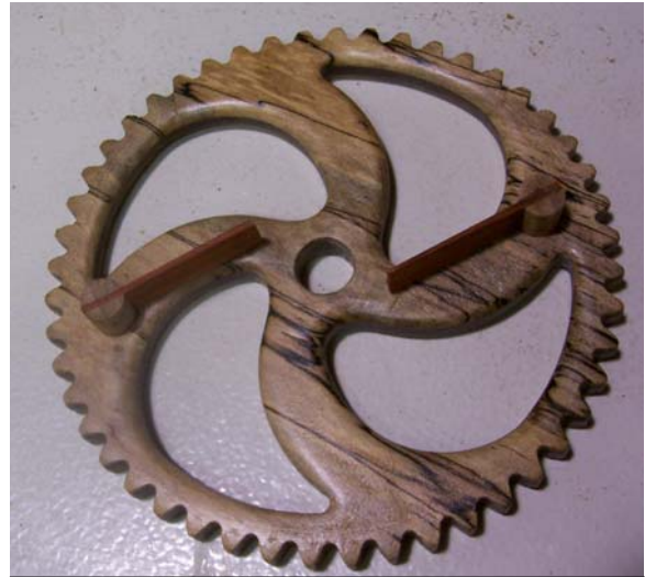
Figure 14 # 39 Pawl Strips are glued in # 40 pawl retainers and Gear # 11
