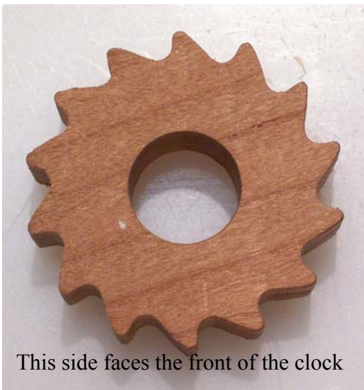
Figure 13 Ratchet is cut from hardwood
