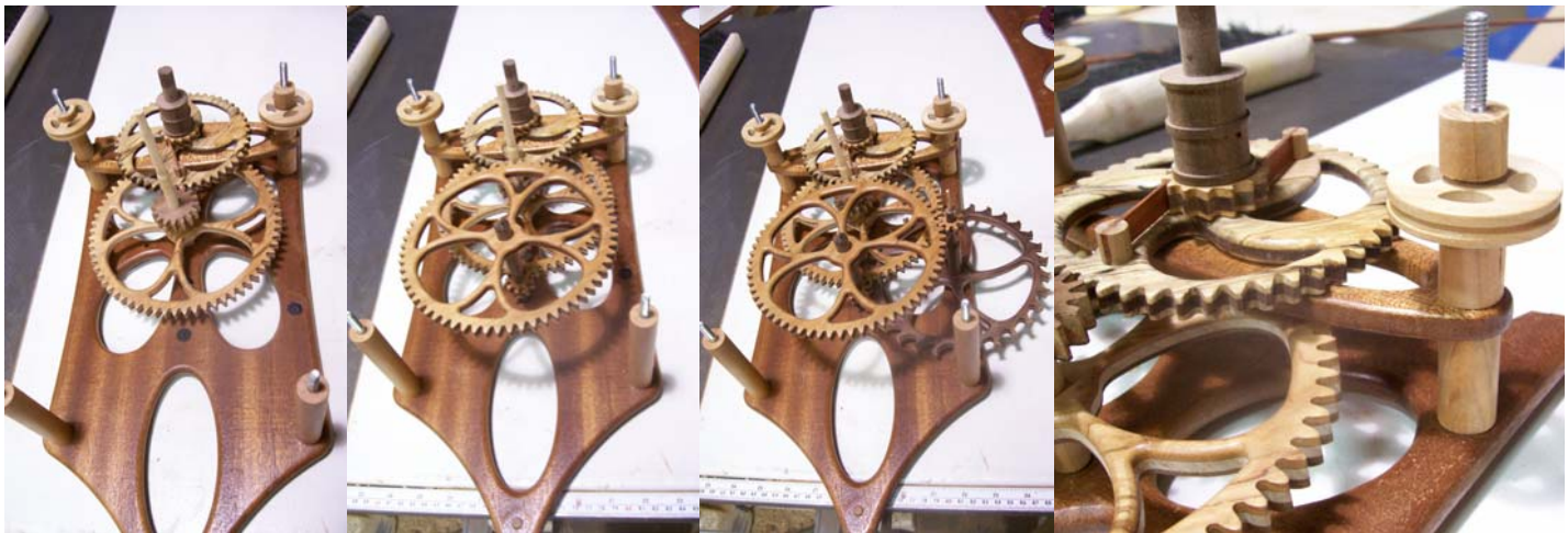
It is easier to assemble the clock by laying it down and adding the parts, then installing the front plate. Do not glue any gears or parts in place until you have dry fitted the parts and are sure they fit properly.
