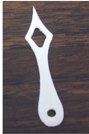
Figure 44 Second hand cut from ivory recycled from an old piano key
