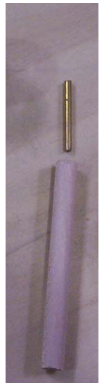
Figure 31. # 20 Escape lever arbor & pin
