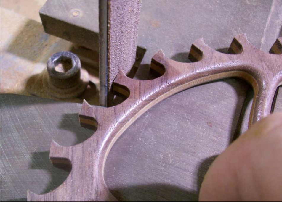
Figure 19 Use a narrow belt sander or sand by hand.
