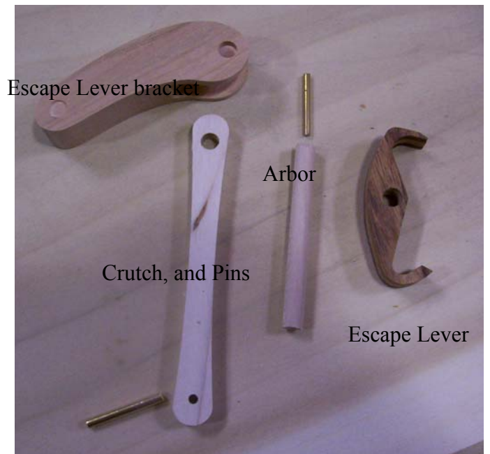
Figure 51 These parts are assembled and control the ticking of the clock.
