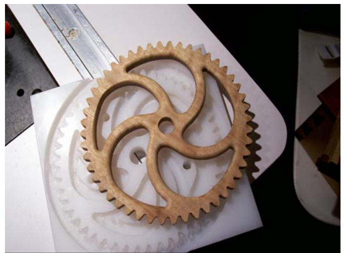
Figure 14 # 10 48 tooth Dial Train gear with spokes rounded ready for sanding and finishing.
