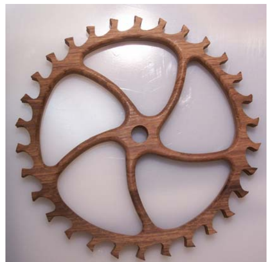
Figure 18 Completed #8 escape gear
