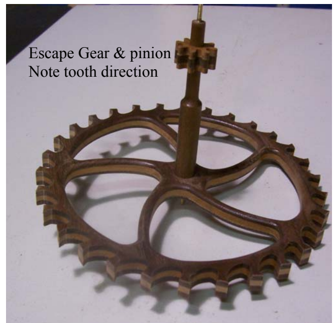
Figure 69 The gear teeth must face the correct direction or clock will not run
