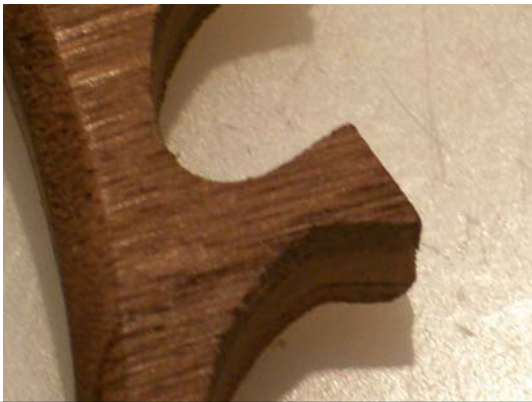
Figure 17 Close up of escape gear teeth
