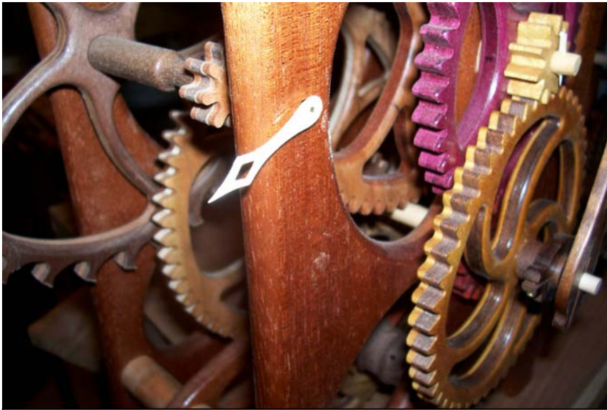
Figure 43 Second hand glued in place after final assembly of clock
