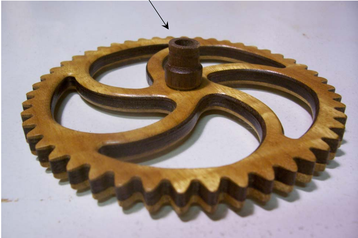
Figure 33 #23 Cannon tube fits into # 48 tooth dial train gear
