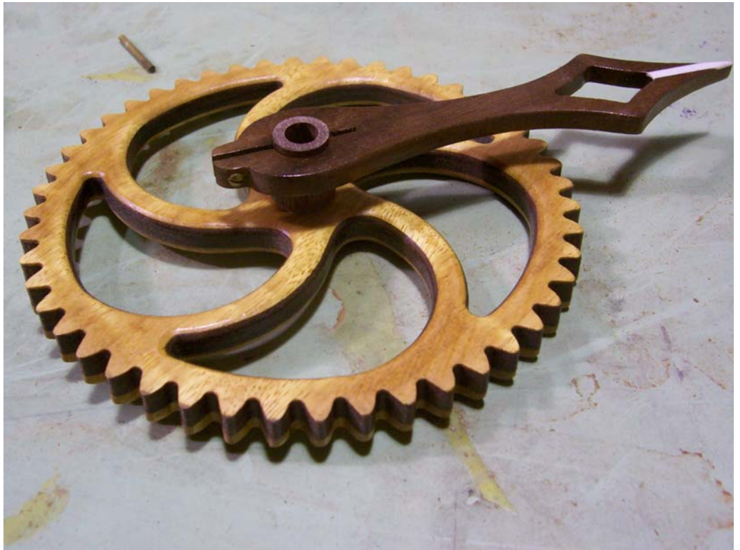
Figure 75 # 10 48 tooth dial train gear with #23 cannon tube and #26 hour hand installed
