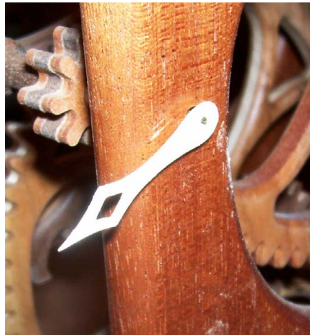
Figure 17 Second hand #27 installed
