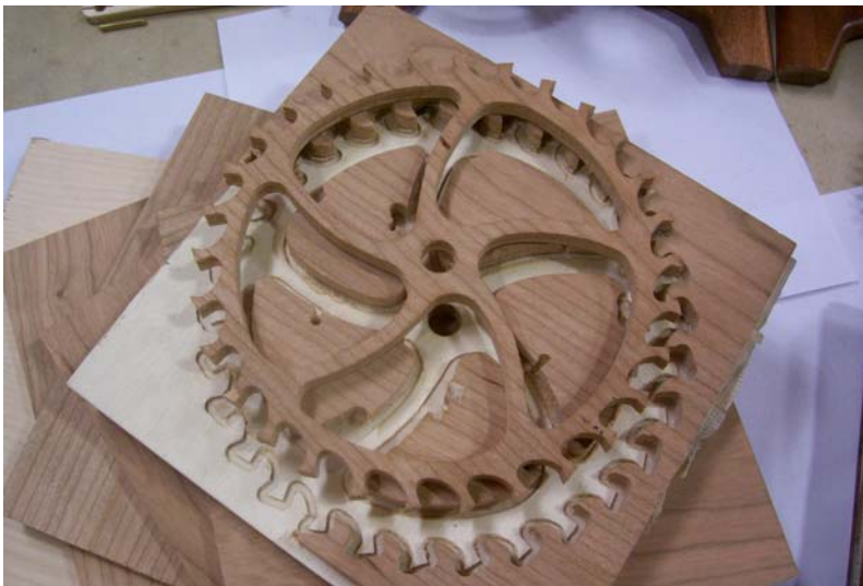
Figure 15 Microwave to remove from backer board
