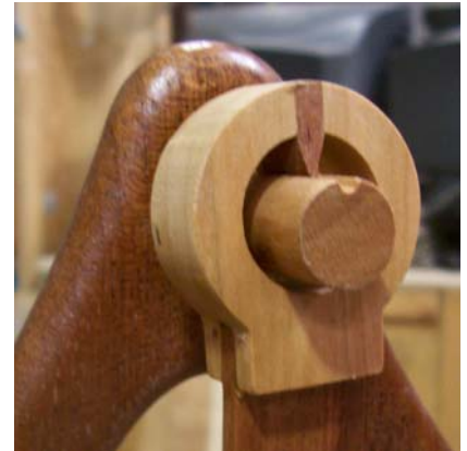
Figure 3 Improved pendulum mount is just one of the reliability improvements of this design
