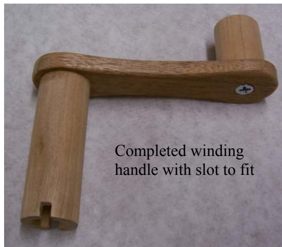
Figure 66 Winding handle must fit the end of the weight arbor
