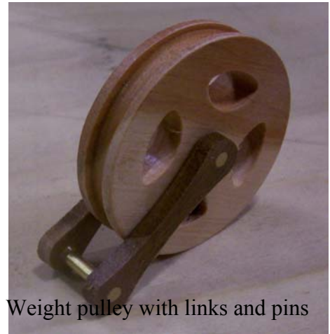
Figure 36 #53 Weight pulleys serve to double length of run time for movement.
