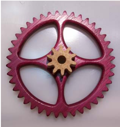
Figure 72 #12 40 tooth gear with #15 10 tooth pinion
