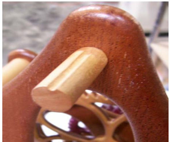
Figure 56 #43 Pendulum hanger mount installed with "V" groove up
