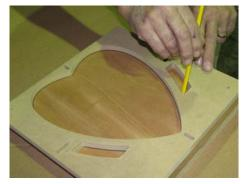
Many Woodline templates feature alignment slots at center locations of the template. These openings allow the template to be aligned precisely. Lay the template on the material and mark the area to be cut with a pencil. Mark the center alignment marks so the template can be replaced in the same position later. When aligning the templates be sure to allow enough space outside the template cut out area for the side of
