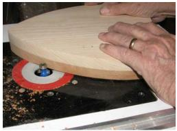
Once the outside is sanded, return to the router table and install a bearing guided round
