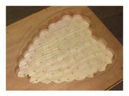
and possibly causing injury. Drill to within about <sup>1</sup>/<sub>4</sub>" but be careful not to drill too close to the edge of the area to be removed. Clean out chips from the drilled out area and inspect. Additional cleanup can be performed with smaller drill bits or a wood chisel if necessary.
