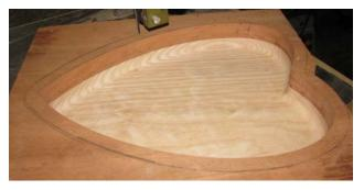
Carefully making these cuts as smooth and as uniform as possible will reduce sanding later.
