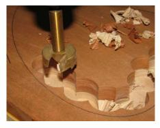
Drill out the area of the template that will form the center area of the tray. Overlap the drilled holes taking care to clamp and hold the material securely to prevent the bit from grabbing the stock
