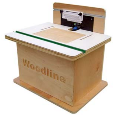
Mustang Router Table with Horizontal attachment mounted and user made wooden insert plate.
