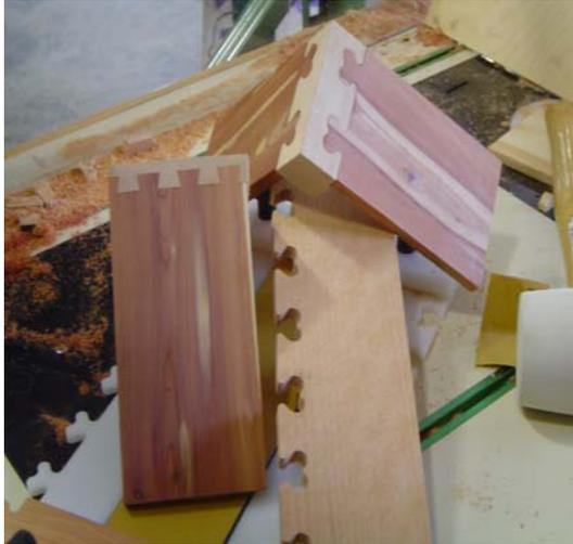
Woodline USA's **Route-R-Joint Junior** system comes with four different joint templates. Interchangeable templates allow switching from one joint to another in just a few easy steps.
