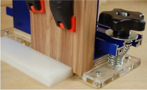
If a flat joint is desired, the mating part can be cut using the pin template in a similar fashion. If a 90° joint is used as shown, install the vertical clamping fence and clamp the material against the fence and up against the end block as shown. Use the gauge block to set the amount of overhang when positioning the vertical fence.
