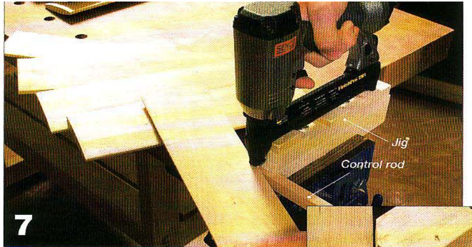
7 Secure the control rod to the jig with a spring clamp. Place each louver at an angle against the jig and over the control rod. Drive a staple into the control rod so that it couples with the existing louver staple (see inset).
