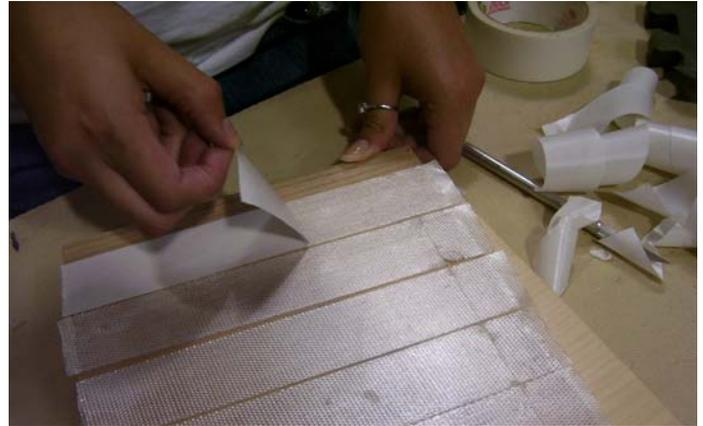
**Figure 4 Use heavy duty double stick tape**
