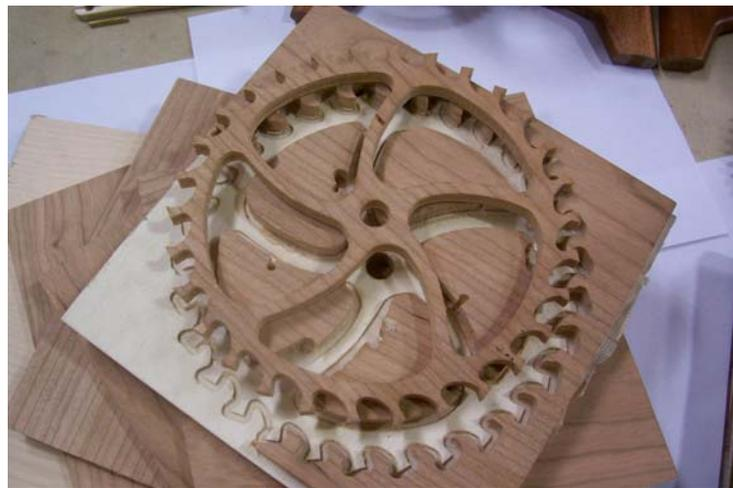
**Figure 3 Microwave to remove from backer board**
