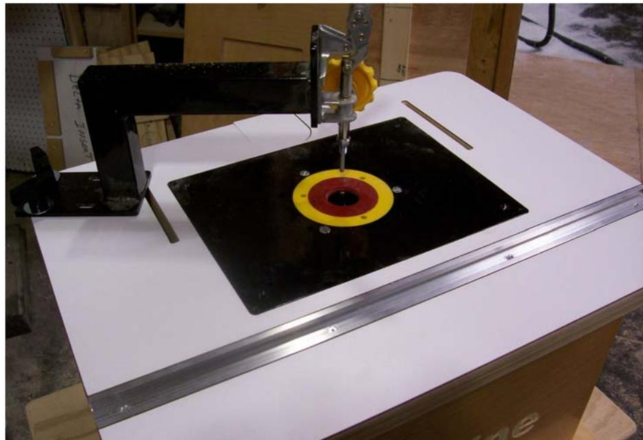
**Figure 2 Pin router can be bolted or clamped to any table**
