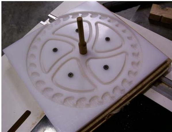
**Figure 5 Gear blank and sacrificial board ready for cutting.**
