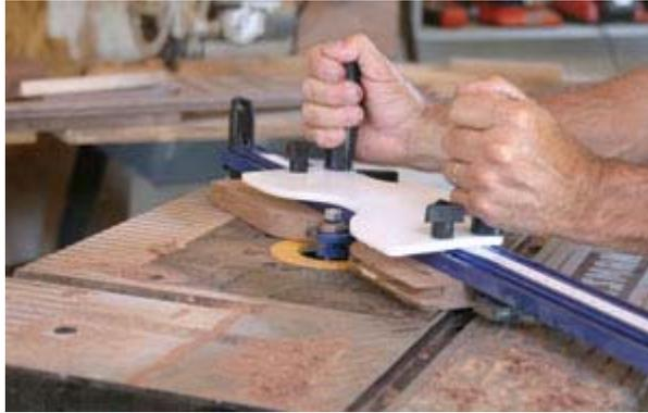
*The jig holds the selected template to match the stock profile and the inside profile cut on the arched rail. Simply guide the jig and stock against the cutter with the handles. A firm grip and steady slow feed rate will result in the best cut.*
