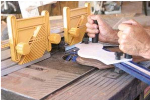
*The holding jig is then used with the reverse side of the template to cut and shape the arched door top.*
