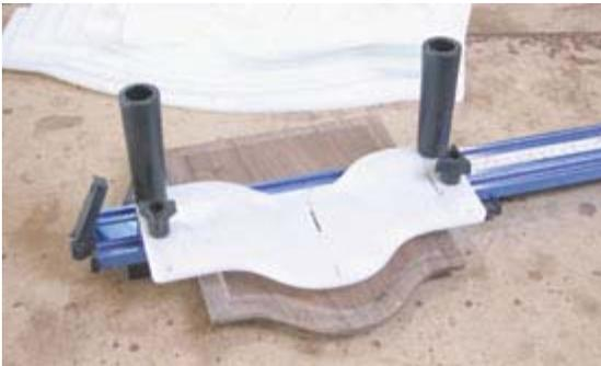
*Woodline has created a unique new Raised Panel Door System that takes a lot of the guesswork and hassle out of the chore. It comes with a set of templates and a jig to hold the template and work stock.*
