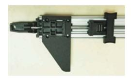
2. Using a small piece of wood, apply pressure to the clamp in order to securely seat the 90 degree head against the clamp pad. Using a C-type clamp, clamp the 90° head to the tool guide. At this time the 90° head should be seated down and against the clamp pad.
