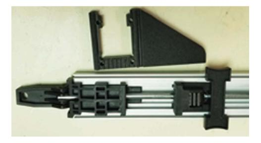
1. Hold the clamp with the bottom side up and install the 90-degree head with the long section to the right and the two ridges in the slots on the rail making sure the 90 degree head is against the black plastic clamp pad.
