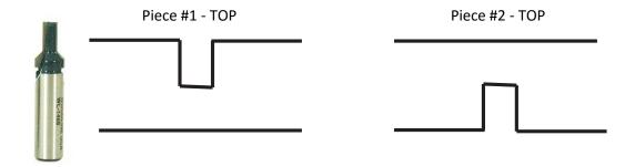
Using the 45° cutter and centering on the dado cuts, cut both sides of both pieces leaving 1/4" material centered between the two angled cuts.
