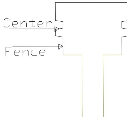
Use glue sparingly. Insert a small bead in each female portion of each board. When clamped the glue will self distribute and make a fine joint.
