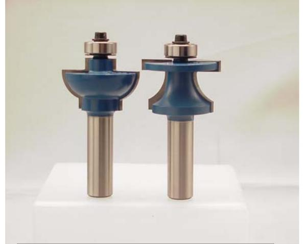
Figure 1. Rail (left) cope cutter
