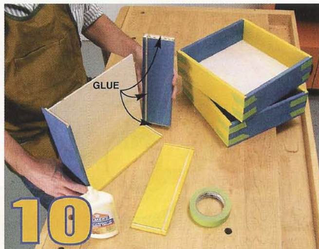
Hold the parts of smaller drawers together with masking tape. Be sure the boxes are square before setting them aside to dry.
