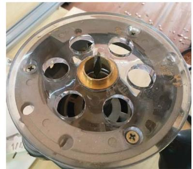
Figure 4 router with 1" bushing installed.
