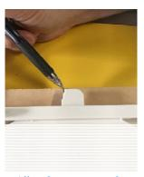
Align the proper notch to match your bit size. 1/4" bit shown.
