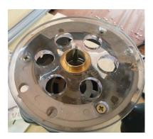
Figure 4 router with 1" bushing installed.
