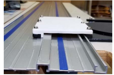
Figure 3 Place over extrusion, loosen all 3 screws, adjust, then tighten.
