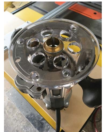
Figure 3 router with 1" bushing installed.
