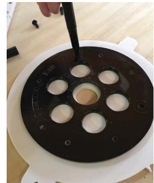
Use the original baseplate to mark the pivot plate.
