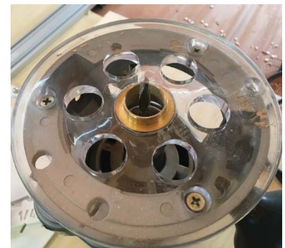
Figure 4 router with 1" bushing installed.
