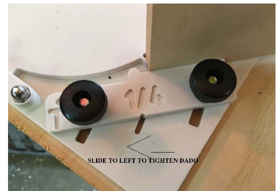
Insert a sample of the wood between the set plate and the pivot plate. Press gently and tighten the knobs snugly. Slide set plate left or right to adjust cut.
