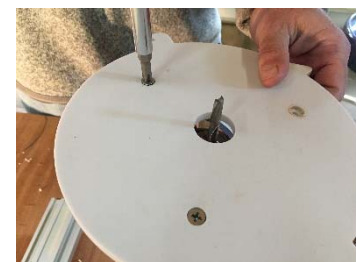
The pivot plate is marked and drilled, then countersunk to fit a router.
