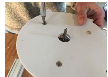
The pivot plate is marked and drilled, then countersunk to fit a router.
