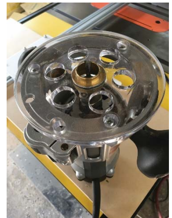
Figure 4 router with 1" bushing installed.
