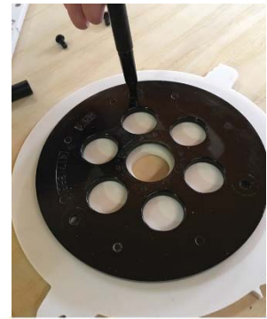
Use the original baseplate to mark the pivot plate.
