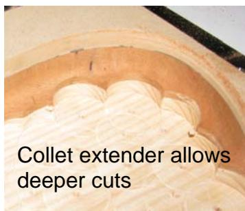
Collet extender allows deeper cuts
