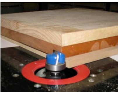
Set bit height. Invert over router table and carefully use multiple passes and clear chips frequently until all tooling marks from drilling operation are removed.
