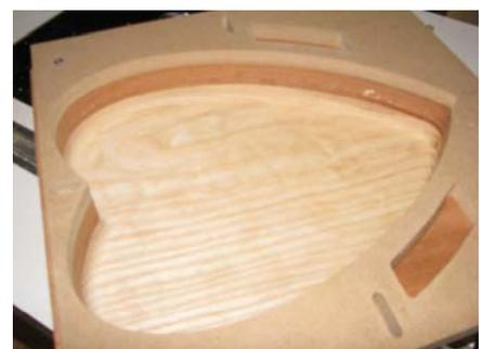
Make a final pass with a light cut and inspect to be sure that all tooling marks are removed and all details are exposed.
