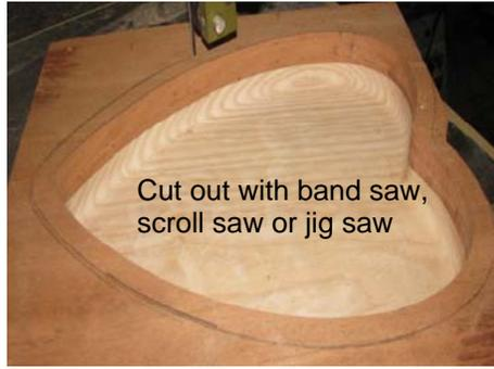
Cut out with band saw, scroll saw or jig saw
