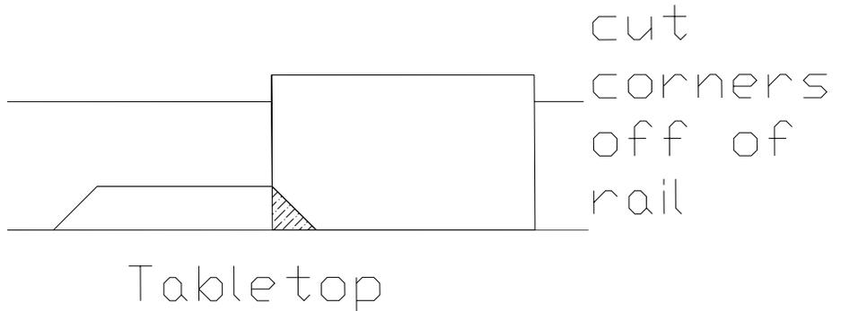
The rails are fastened to the stile with glue and pocket hole screws from behind. Be careful not to use so much glue that it gets in the beaded portion, where it will become difficult to clean out.
