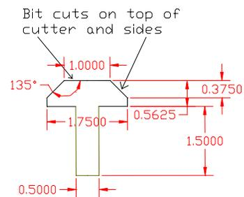
face frame can be any width but a dividing rail such as a divider between drawers, must be a minimum of 1 1/2 inches wide. With a simple jig beaded face frames are quick and simple to produce on any standard router table.
