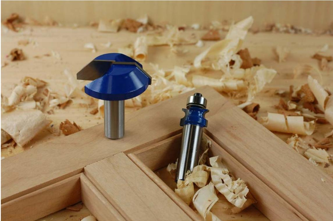
The 1460S/MD530 beaded face frame set consists of two matched router bits. One bit cuts the bead, and the second bit miteres the joint where the bead meets in the corner of a face frame. Edges of
