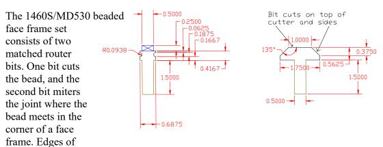
face frame can be any width but a dividing rail such as a divider between drawers, must be a minimum of  $1\ 1/2$  inches wide. With a simple jig beaded face frames are quick and simple to produce on any standard router table.
