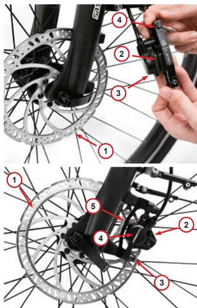
**Note:** when fixing the Disc brake bolt, drag the lower part of the Disc brake with hand, and push the Disc brake upward as far as possible.
