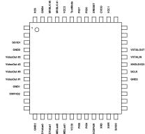
Figure 1: LQFP48 pin out (not to scale)
