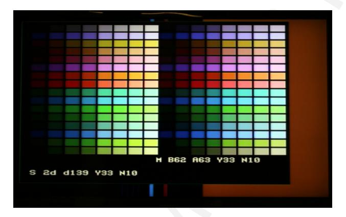
The large span of variation in the color coefficients results in a nice spread of different hues, which are useful for bright user interfaces, games, animations and such. Also a lot of darker tones are available. The first 8 values form a very near grayscale. The next 8 values have a slightly bluish tone and the last 8 values form a grayscale with a seepia tone.
