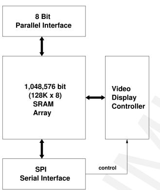
Figure 2: SPI or 8-bit parallel interface and Video Display Controller can be enabled at the same time.
