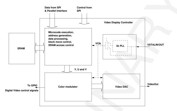
Figure 5: Video Display Controller block diagram
