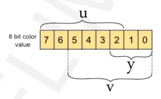
This assignment strategy takes, from the 8-bit pixel color value, 6 bits to u color coefficient, 6 bits to v color coefficient and 3 bits to luminance. That results in a large amount of different hues and also dark and bright luminances for most colors.
