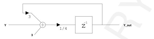
Figure 7: Switchable low-pass Y filter
