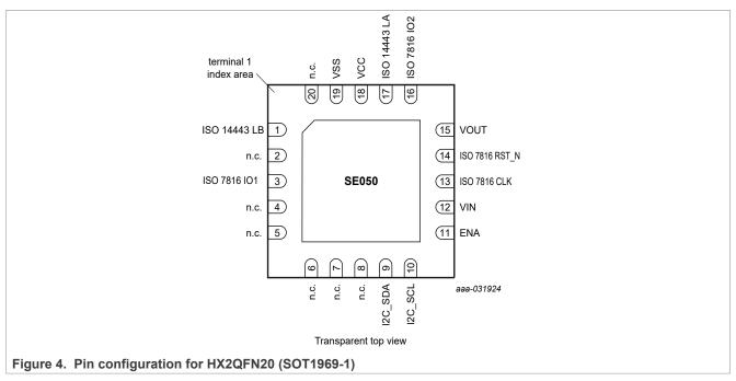
**Note:** Terminal 1 index area is marked on the bottom with a notch on the center pad and on the top with a printed dot.
