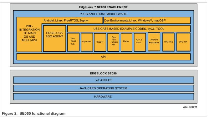
The SE050 uses I<sup>2</sup>C as communication interface. <u>Section 4</u> gives more details. The SE050 commands are wrapped using the Smartcard T=1 over I<sup>2</sup>C (T=10 I2C) protocol. The detailed documentation of the SE050 commands (see [3]) and T=1 over I2C protocol encapsulation is available on [1].
