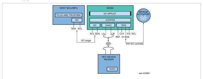
Figure 1. SE050 solution block diagram
