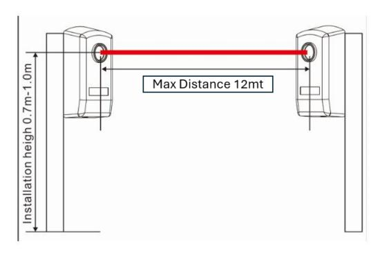
The safety beams are suitable for single or double gates. The transmission (TX) beam can be run off battery or hard wired. If you intend to hard wire the TX beam, run the supplied 2 core cable
