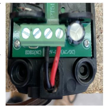
Wire the supplied 5 core cable into the receiving (RX) beam.
