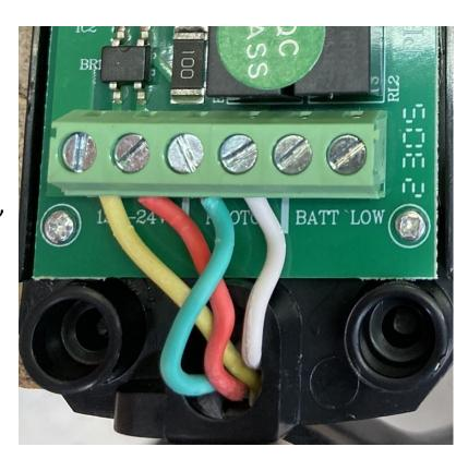
Run the 5 core cable and the 2 core cable into the control box. Cut off any excess. The wiring to the board is as follows: 5 core Red & 2 core Red to Positive(+), 5 core Yellow & 2 core Black to Negative(-), 5 core white to COM, 5 core Green to Photo Electric Beam.
