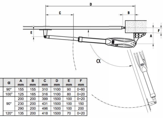
The mount distance for the drive unit and the hinge distance for the gate can be selected to optimise the side room clearance.
